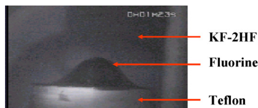
Fig. 3. Fluorine bubble generated in \text{KF}-2\text{HF} on a horizontal electrode facing the top of the electrochemical cell. Reprinted from ref. [43].
